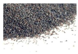
We manufacture BFA in tilting furnace or fixed furnace, Tilting Furnace BFA has higher Al2O3 content, lower impurities and high-performance.
